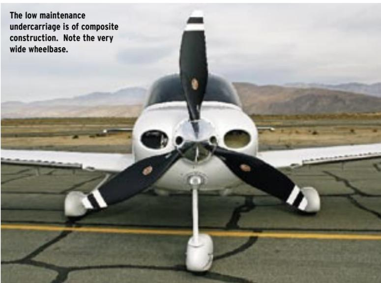
The low maintenance undercarriage is of composite construction. Note the very wide wheelbase.
