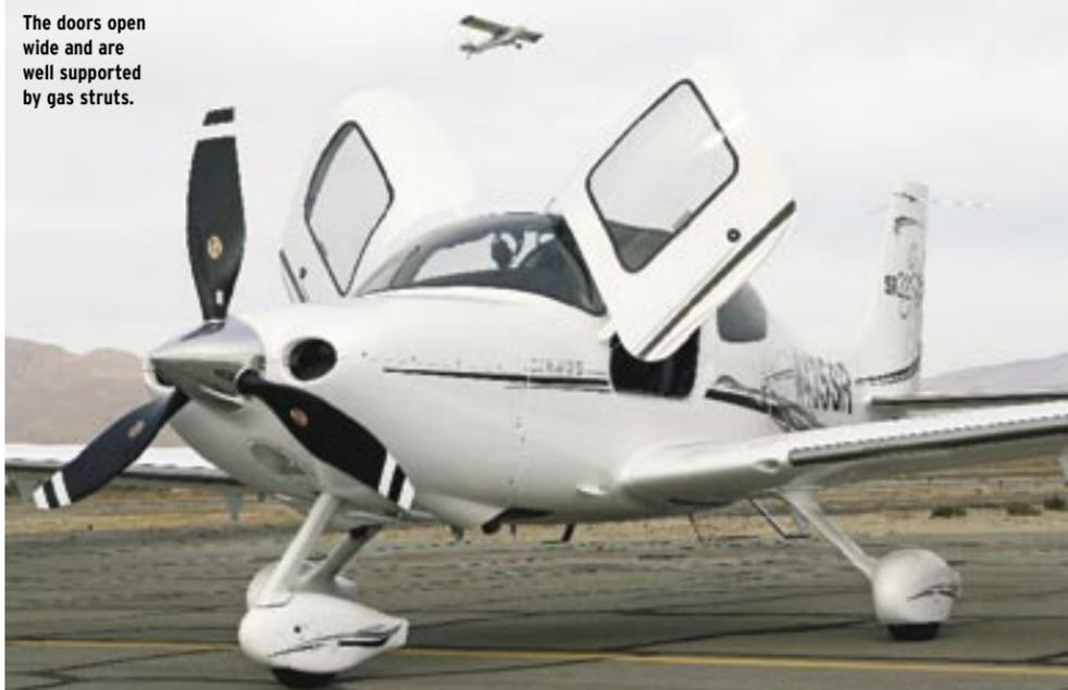
The doors open wide and are well supported by gas struts.
