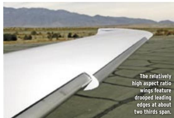
The relatively high aspect ratio wings feature drooped leading edges at about two thirds span.
