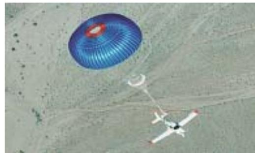
**The Cirrus Airframe Parachute System (CAPS) is unique in a production light aircraft. This series of shots shows the system deploying from its hatch in the cabin roof after being fired by a handle-activated solid fuel rocket.**
