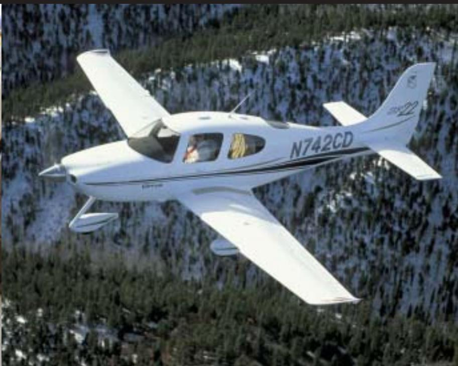
SR20 is the fact that despite its fixed undercarriage, its maximum cruising speed of 160kt (296km/h) is some 20kt (37km/h) faster than the similarly powered, narrower cabin and retractable Piper Arrow.
