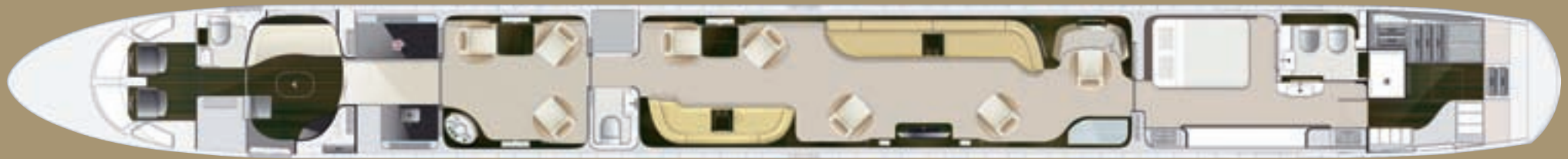
Optional floor plan with stand-up shower. 4,085 cubic feet (115.7 cubic meters) of cabin volume in five distinct privacy zones.
